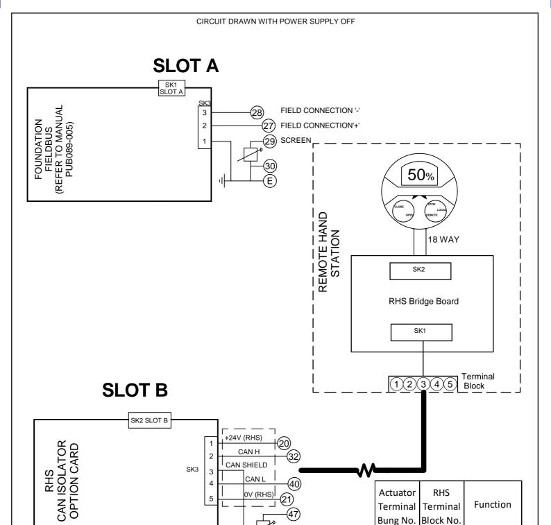
RHS CABLE IS CUSTOMER SUPPLIED, FOR SPECIFICATION SEE PUB002-059, MAXIMUM LENGTH OF CABLE TO BBE 100m.
