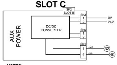
SUPPLY FROM SK11 ON MOTOR CONTROL PCB
