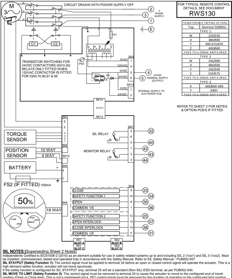
position (Open or Close limit). This is not a maintained input, SF2 control signal must be removed for the duration of operation to the configured limit position. This is a low demand safety function. If the safety function is configured for SIL MOVE TO LIMIT (SF2) ONLY, terminal 34 will be a standard Stop/Maintain input in accordance with PUB002-041.
