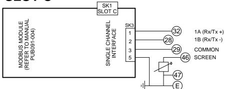
PASSIVE TERMINATION CONTROLLED VIA SETTING IN ACTUATOR CONFIGURATION. REFER TO PUB002-040
