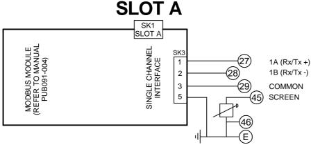
PASSIVE TERMINATION CONTROLLED VIA SETTING IN ACTUATOR CONFIGURATION. REFER TO PUB002-040
