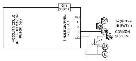
PASSIVE CONTROLLED VIA SETTING IN ACTUATOR CONFIGURATION. REFER TO PUB002-040
