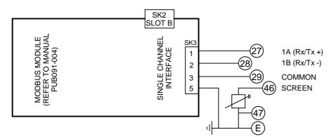
MODBUS INPUT FOR CLC SETPOINT (CONTROL SOURCE 1)
