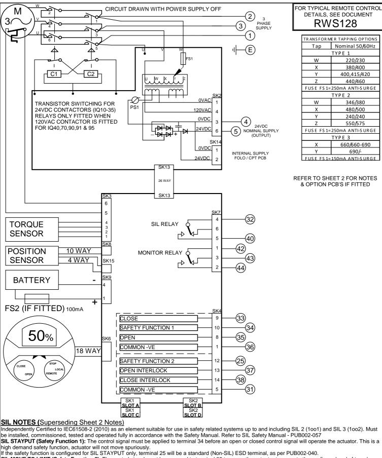
Independently Certified to IEC61508-2 (2010) as an element suitable for use in safety related systems up to and including SIL 2 (1001) and SIL 3 (1002). Must
