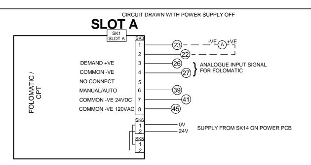
FOR MANUAL/AUTO CONNECTIONS AND DETAILS OF FOLOMATIC/CPT FUNCTIONS REFER TO ROTORK PUBLICATION PUB002-041 FOR PAKSCAN CONTROL FOLOMATIC MUST BE CONFIGURED FOR MANUAL OPERATION
