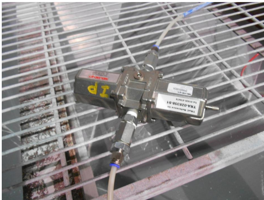
SPECIMEN BEFORE UNDERGOING IP6X DUST TEST
