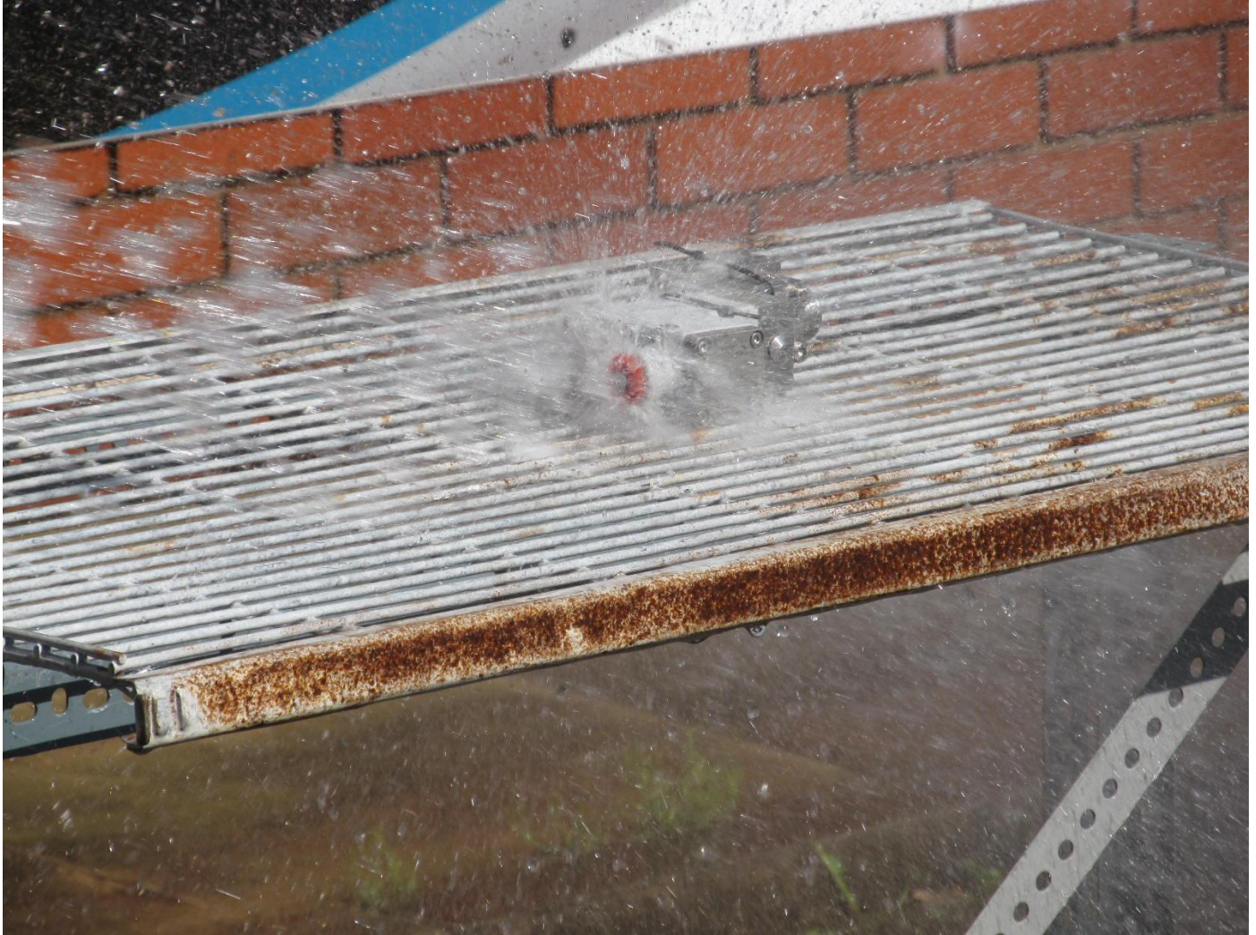
SPECIMEN UNDERGOING IPX6 POWERFUL WATER JETTING
