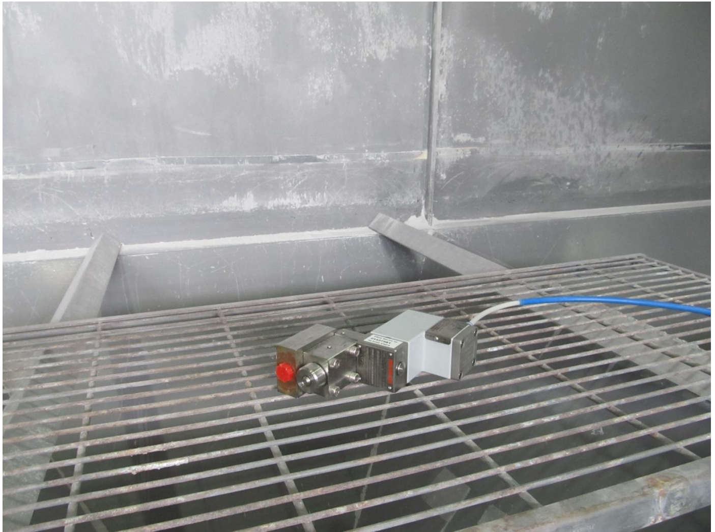
SPECIMEN SETUP FOR IP6X DUST INGRESS TESTING
