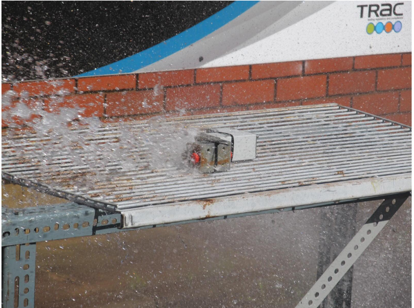
SPECIMEN UNDERGOING IPX6 POWERFUL WATER JETTING
