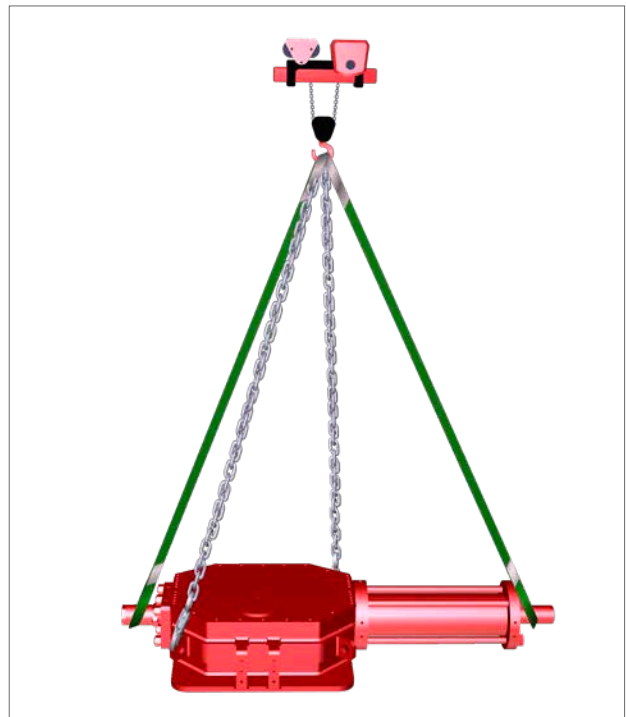
Fig 7.4 Lifting (double-acting actuator size 200 - 350)
