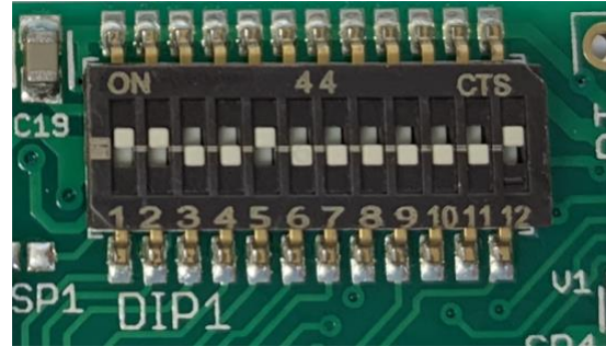
In this example DIPs 1, 2, 5 and 12 are on.
