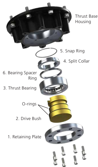
Fig. 5.1.4 F25 & F30 base assembly
