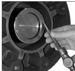
Fig. 4.6 Removal of Retainer
