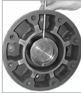
Fig. 4.12 Tightening Retainer Set Screw
