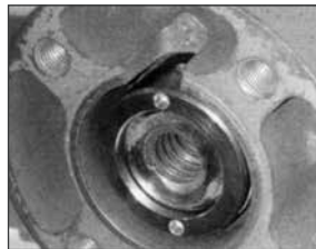
Fig. 4.8 Type A Drive Bush in Position 1
