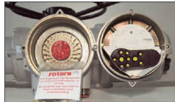
Fig. 6.1 - Actuator containing Rotork actuator setting tool.
