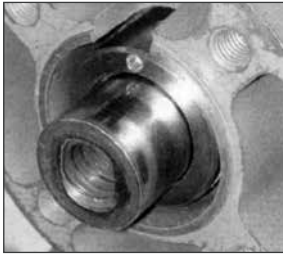
Fig. 4.9 Type A Drive Bush in Position 2
