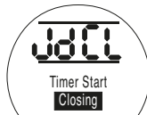
Pulsed Operation Around the Closed Position
