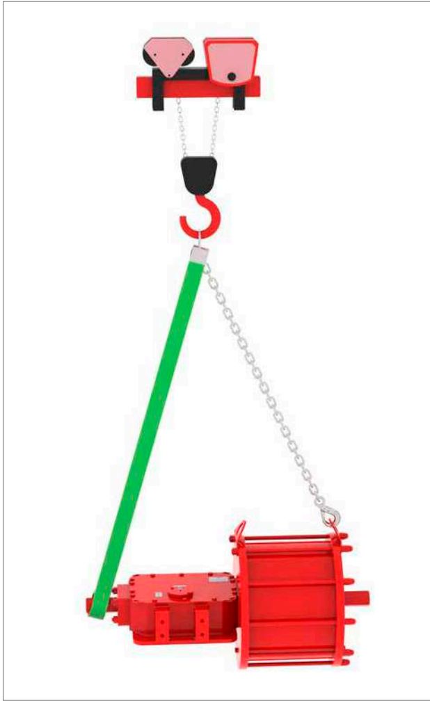
Fig 7.2 Lifting (double-acting actuator up to size 130)
