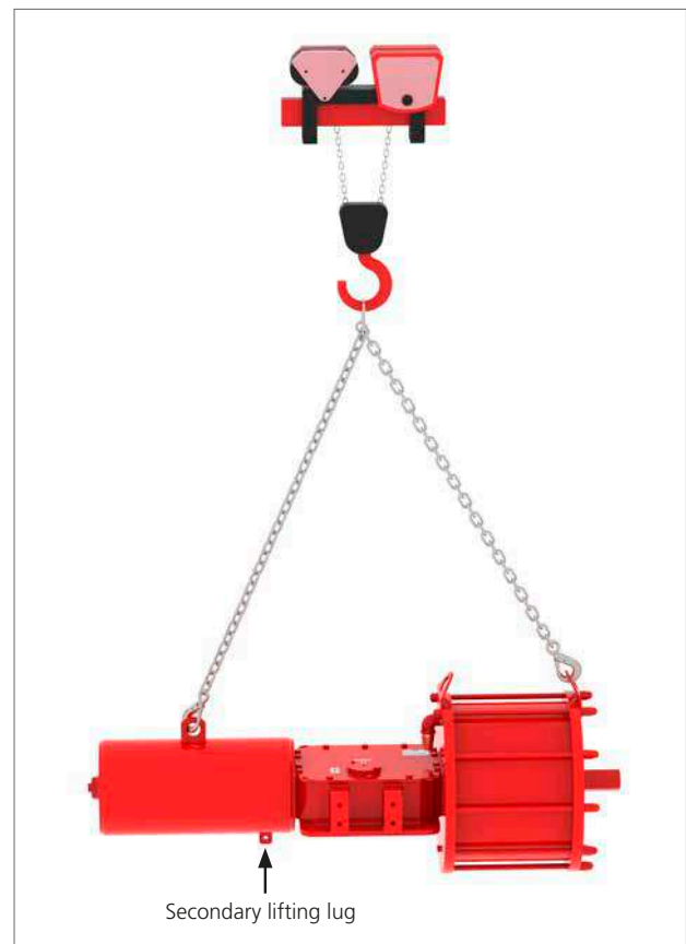
Fig 7.1 Lifting (single-acting actuator up to size 130)
