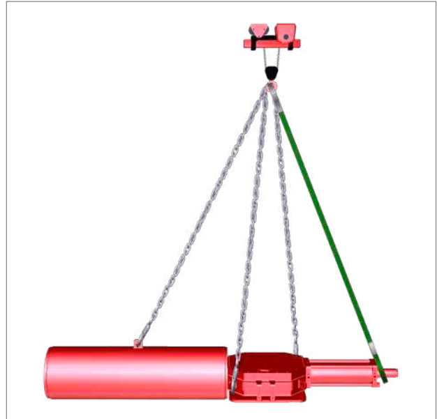
Fig 7.3 Lifting (single-acting actuator size 200 - 350)
