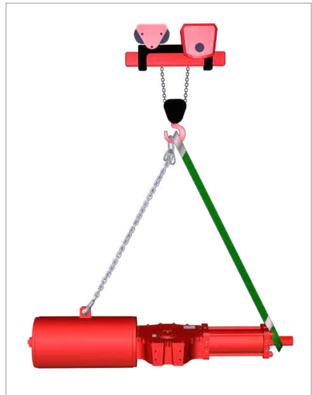
Fig 7.1 Lifting (single-acting actuator up to size 161)
