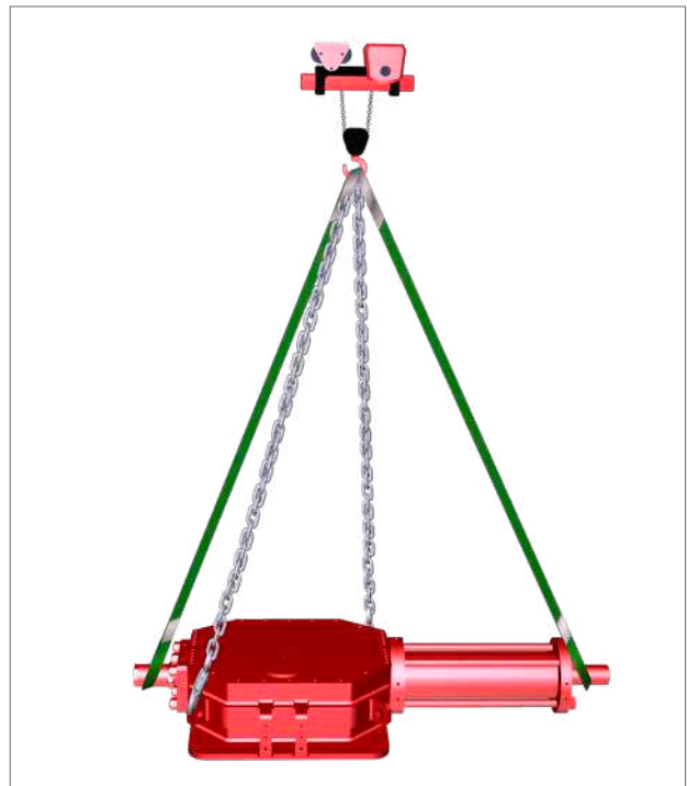
Fig 7.4 Lifting (double-acting actuator size 200 - 350)
