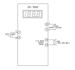
Due to wide variations in the terminal numbering of actuator products, actual wiring should follow the print supplied with the control station.
