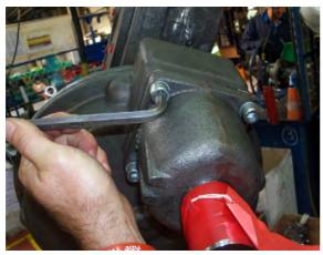
1. Remove the four SCM12X30 cap screws using a 10mm Allen key.
