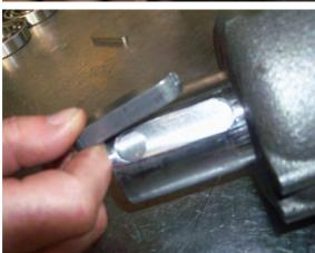
3. Remove the key from the shaft – to allow the extraction of the shaft, 2 bearings and 1 spacer.
