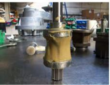
7. Ensure that the O ring on the flange face and the flange seat are intact – and smear a small amount of grease on the surface. This will allow the shaft to pass through the O ring without damaging it – and will help the flange to fit back into the gearcase.
