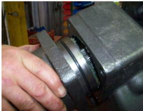
2. Remove the flange from the gearcase.
