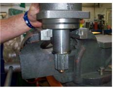
5. Remove the outer bearing by hand. In the event that the bearing is tight – use a suitable drift and tap the bearing through the front face of the flange. Then remove the spacer and clean out the flange cavity of residual grease. This will then reveal the inner bearing which can also be removed in the same manner as the outer one.
