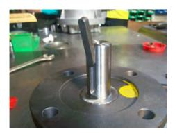
Re-fit the new key onto the shaft and gently tap into position wiping away any excess grease from the base of the shaft.
