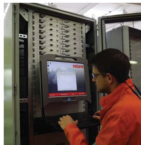
The Smart Valve Monitor (SVM) is an advanced partial stroke test and monitoring system for ESD valves. This centralised control cabinet will be installed at a UK gas import plant.
